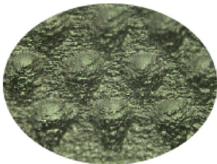
Fig. 12 Texture characteristics of discharge chamber at 50X with optical 3D profiler (partial)
