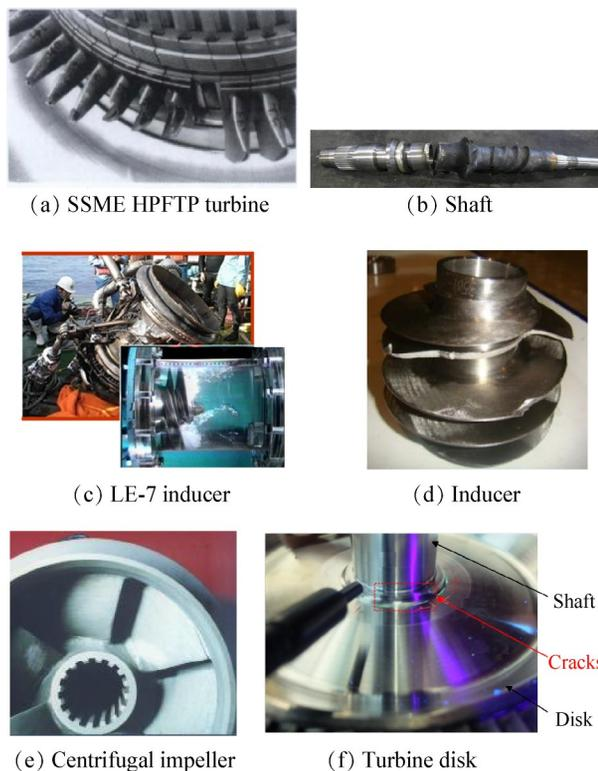
Fig. 8 Typical faults of turbo-pumps
