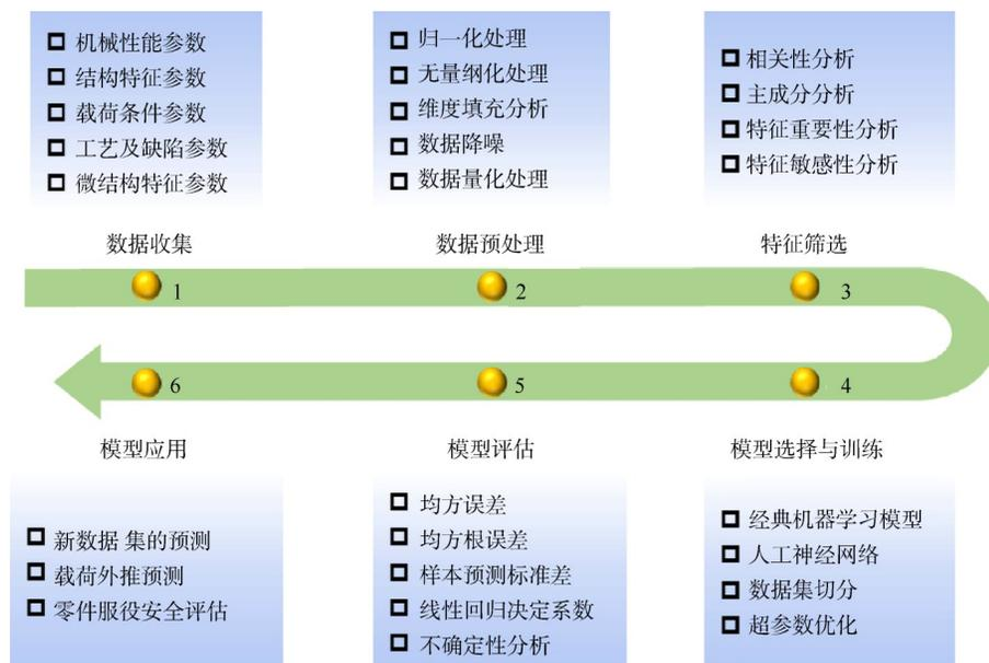
Fig. 5 Machine learning based life prediction process
