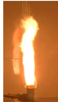
**Fig. 6 Combustion of propellant samples at atmospheric pressure**
