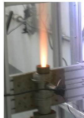
**Fig. 8 Tester test of ultra-high burning rate propellant embedded with porous spherical particles**
