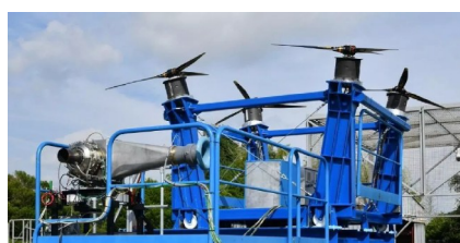
Fig. 8 100kW hybrid system of Safran [38]
