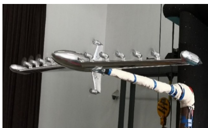
Fig. 9 Tailstock hybrid distributed propulsion scheme and wind tunnel test [45]
