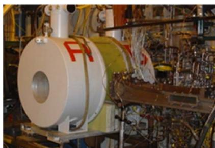
(c) Assembled scramjet MHD test bed
