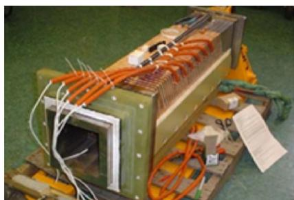
(b) Assembled MHD generator channel
