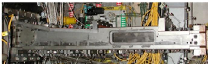
(a) UTRC test Cell 5 scramjet test article
