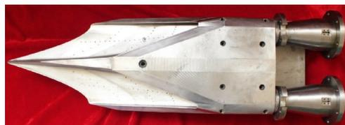
Fig. 4 Test model of the bimodule inward turning inlet
