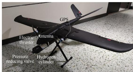
Fig. 2 Physical picture of UAV
