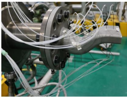
Fig. 6 Serpentine exhaust experimental setup and its surface pressure taps distributions
