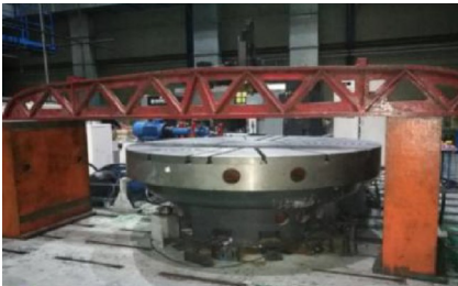
Fig. 15 Q1-205 new type hydrostatic bearing test bench
