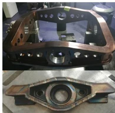
Fig. 18 Gimbal ring/beam after hot-fire test using AM technology
