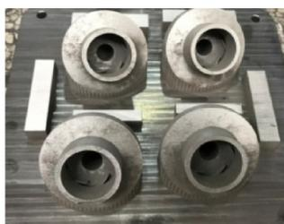
(a) Y/R turbine impeller
