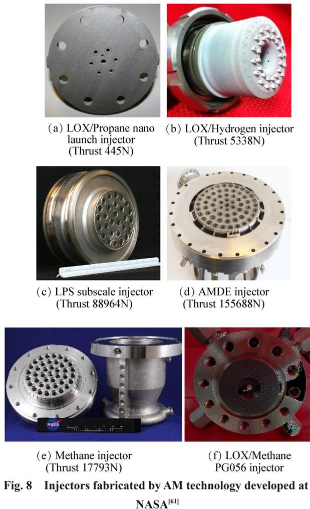
Fig. 8 Injectors fabricated by AM technology developed at NASA<sup>[61]</sup>
