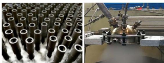
(a) Injector shape (b) Injector flow test
