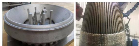
(a) Nozzle manufactured by SLM technology (b) Nozzle manufactured by LWDC technology
