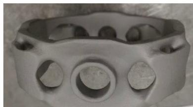
Fig. 17 Gimbal ring after topology optimization using AM technology
