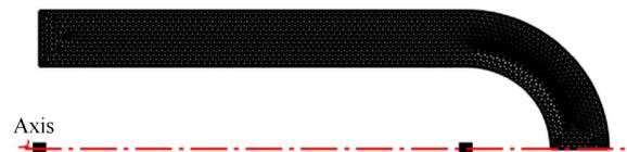
Fig. 5 Unstructured grid of PCM cavity
