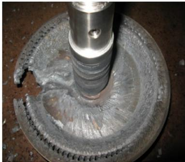
Fig. 13 Burning of turbine rotor
