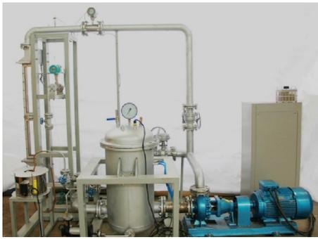
Fig. 6 Picture of experimental system of flow condensation for gas-liquid two phase
