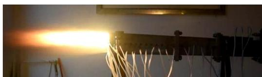
Fig. 16 Flame image at the outlet of combustor
