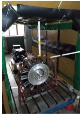
Fig. 1 Fan blade foreign object impact test platform
