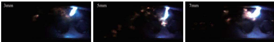
Fig. 12 Ignition process of plasma igniter at 6.0ms varying with anode channel length
