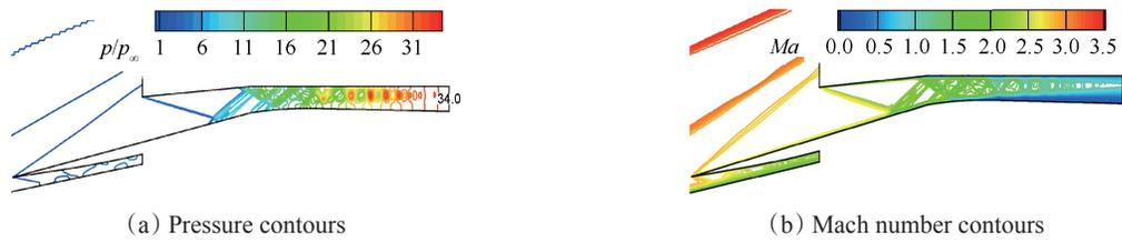
Fig. 10 Flow field of inlet after adjustment in critical status at  $Ma_\infty = 3.5$
