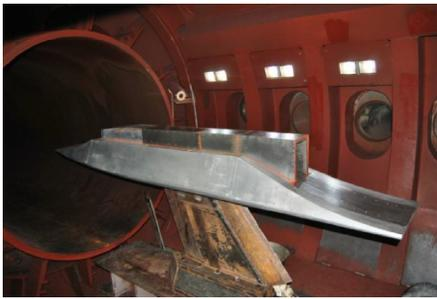
Fig. 9 Free jet test model for airframe-propulsion integrated vehicle
