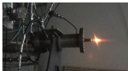
Fig.6 Torch igniter in testing
